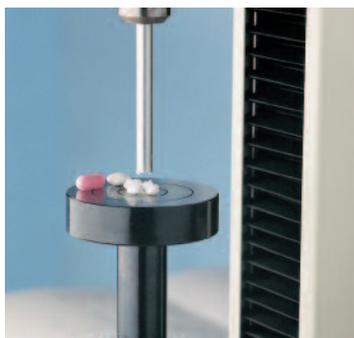
**Fig 15.** Testing the crushing strength of pills
