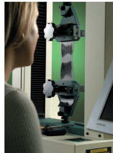
**Fig 32.** Tear test on rubber specimens using S453 grips
