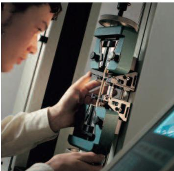
**Fig 25.** Reinforced plastic dumbbell samples
