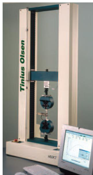
**Fig 37.** Model H50kT with HT21 grips
