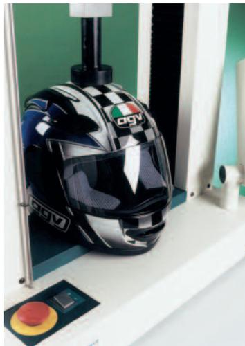
**Fig 27.** Compression test on crash helmet
