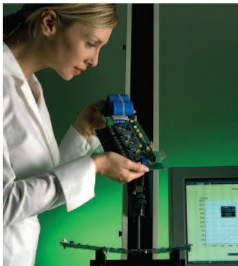
**Fig 7.** Model H5kT being used to determine the flexural strength of a printed circuit board
