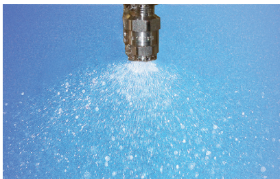
Outdoor moisture attack is simulated by spraying pure water onto specimens.
