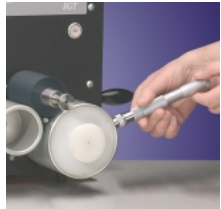
Applying ink with the IGT ink pipette
