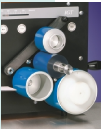
Inking the printing disc
