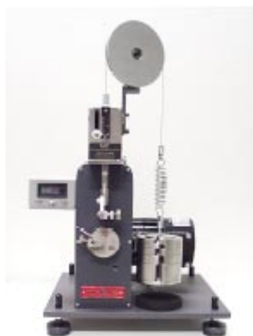
Figure TD 909-1. Model 1 Folding endurance tester for paper with optional exhaust fan for testing in accordance with ASTM D2176 and TAPPI T-511.
