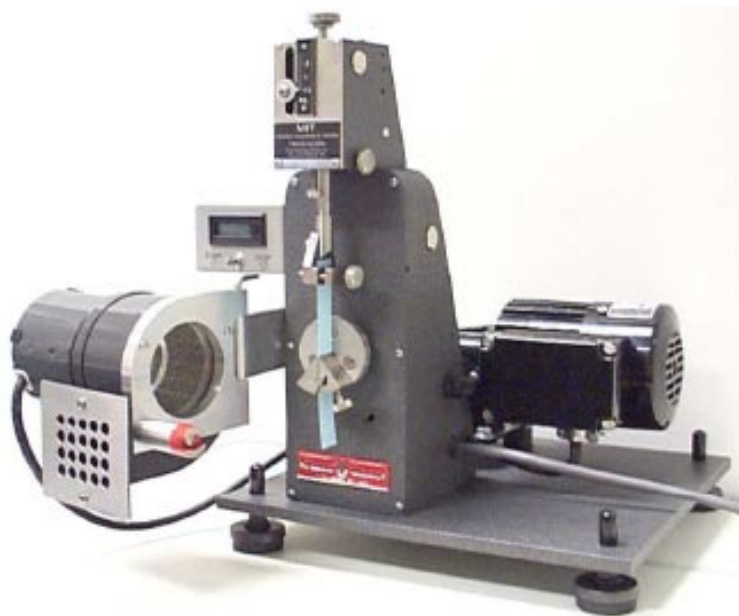
Fig. TD 909-2. Model 2 Folding Endurance Tester with modified loading system and digital counter is for use on materials with relatively high amounts on elongation.
