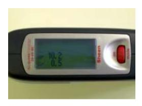
Basic mode – For a single measurement of gloss at the selected geometry - the basic mode gives quick snapshot information which is displayed on screen.
