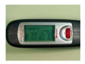
Sample mode – Allows measurements to be taken and referenced to a standard value which is assigned by the user. On screen information indicates the difference between the sample and the standard.
