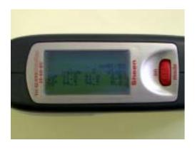
All measurements are made at the same location on the sample no matter which measurement geometry or geometries are selected. The results are displayed instantly – including difference, Pass / Fail and Statistics.
