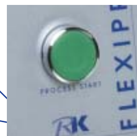
Dual start buttons for safety
