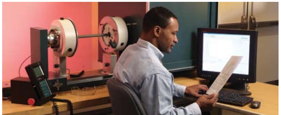
Fig 2. Bench mounted 10,000 in.lbf machine.
