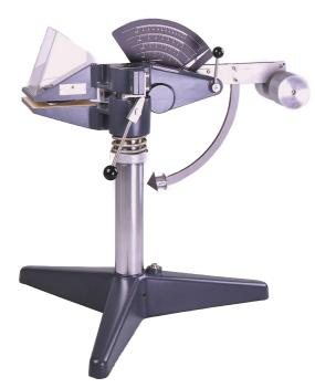
The Puncture Tester is designed to measure the energy required to puncture corrugated board and therefore help assess the protective qualities of that board. In addition to the risk of damage from transport and stacking there is the potential of being struck by sharp objects.
