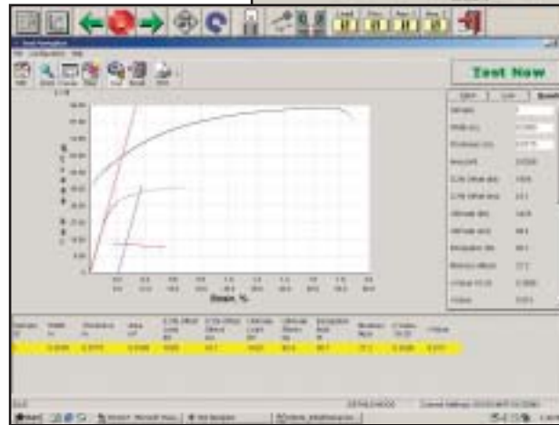
Fig. 8. Completed test with a complete test result, with r value; note that the extensometer stays on the sample until break
