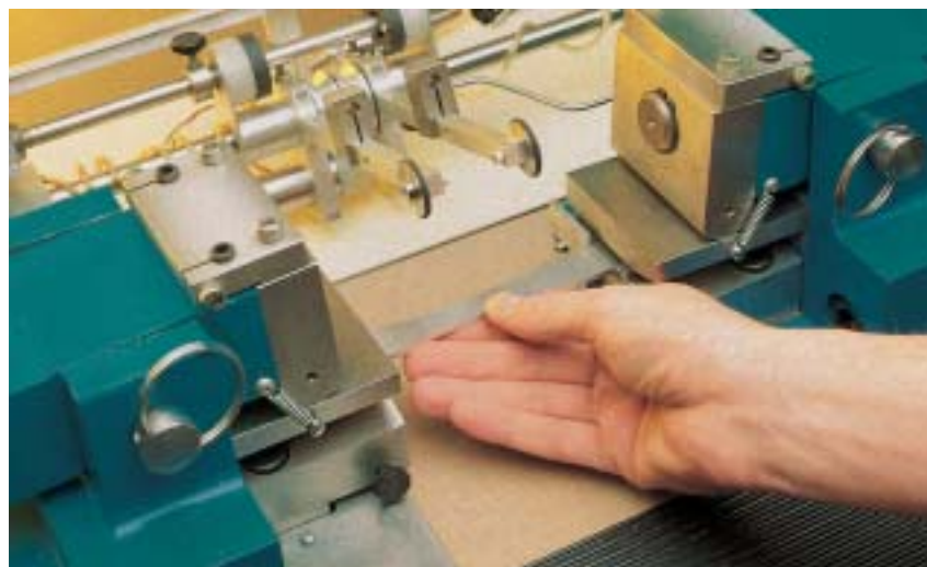
Fig. 3. Close up of unique extensometer that can stay on to sample fracture. The sample is loaded against the mechanical stops and the test started — the rest is automatic
