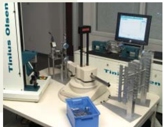
Fig. 6. Detail showing the pick-and-place robot, sample racks, laser barcode reader, and sample dimension measuring station, broken sample bin, and another test station. This second test station could be a flexure test, a hardness test, or another kind of physical test
