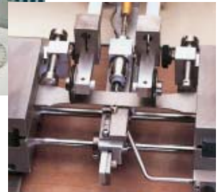
Fig. 4. Optional r value instrumentation on computer controlled extensometer allows fast, accurate r value calculations
