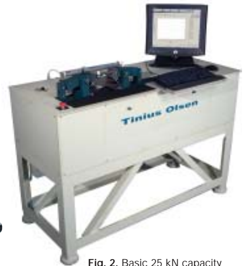
Fig. 2. Basic 25 kN capacity horizontal tensile testing machine, shown with optional extensometer
