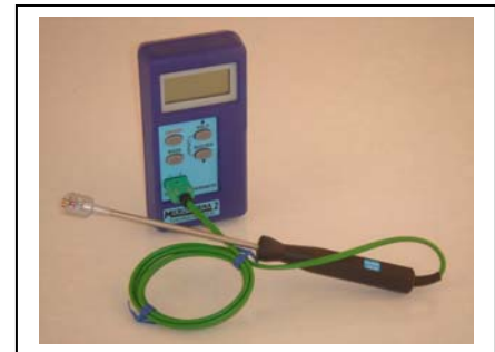
Thermometer and s/s band surface probe to check jaw temperatures.
