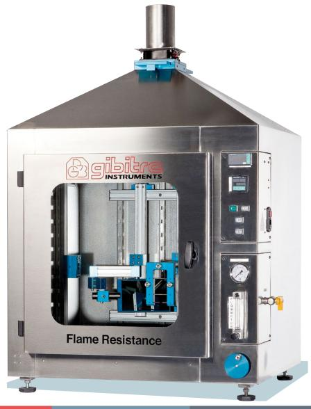
Laboratory instruments for rubber and plastic testing UL 94, ASTM D 4986 and equivalent standards.
