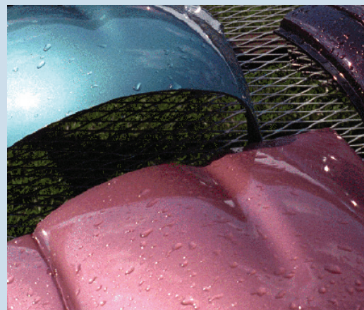
Using a unique condensation mechanism, the QUV reproduces dew, the main cause of outdoor wetness.
